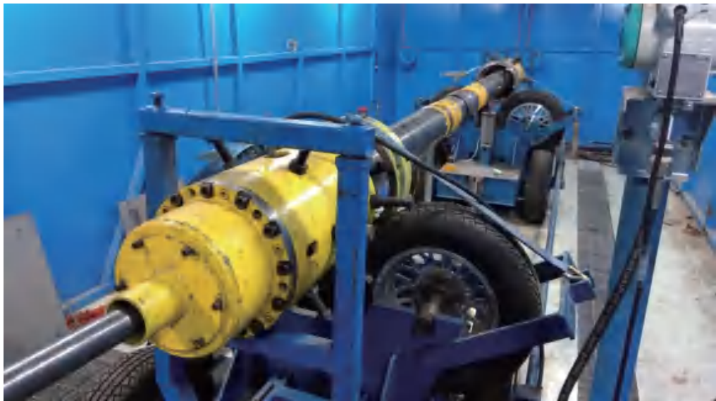
Figure 4 Full scale fatigue test
