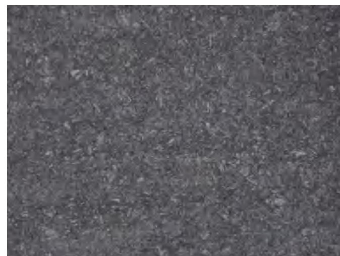
Photo Tempered Macrostructure of TP155V (x500)
